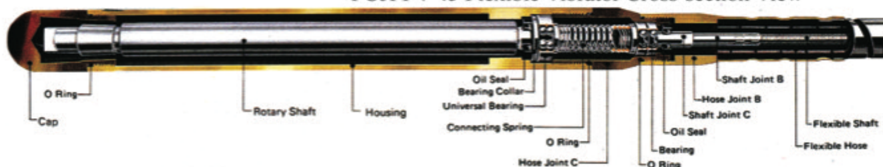
FUJI FV 45 Flexible Vibrator Cross-section View
