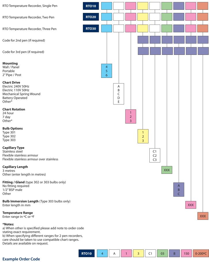
Single pen temperature recorder, wall mounted, electrical 240 volt 50hz chart drive, 24 hour rotation, non-toxic Type 303 bulb, 3 metres of stainless steel capillary, immersion length 150 mm, 1/2" BSP male fitting, , range 0 to 200 Deg C.
