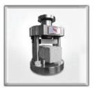
Mortar Prism Compression Device
