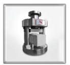
Mortar Prism Compression Device
